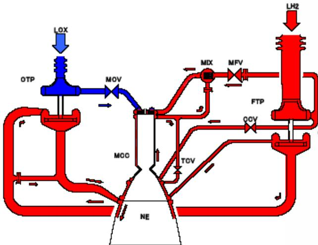
Fig. 2 LE-X engine cycle
