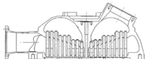
Fig. 6 LE-X injector
