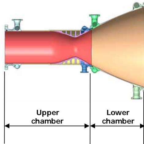
Fig. 5 LE-X combustion chamber
