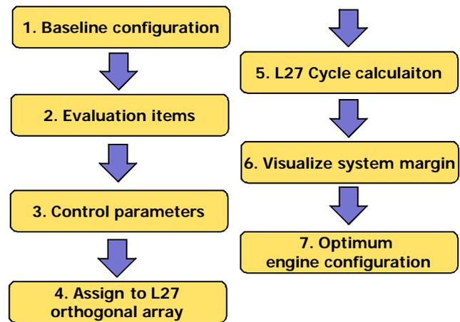
Fig. 3 Design process of optimization
