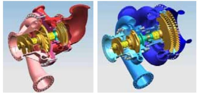
Fig. 9 LE-X engine turbopump (Left :FTP / Right :OTP)
