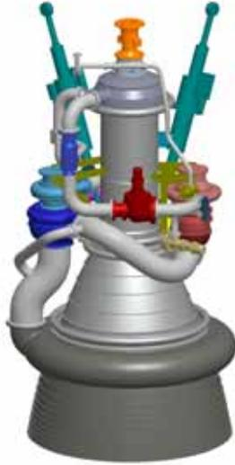
Fig. 4 LE-X engine 3D layout model
