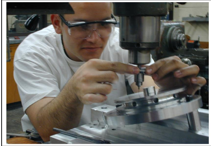
***Figure 7-Drilling of injector holes***
